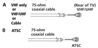
Use option A to connect the TV to a cable system or an antenna with a 75-ohm cable.
